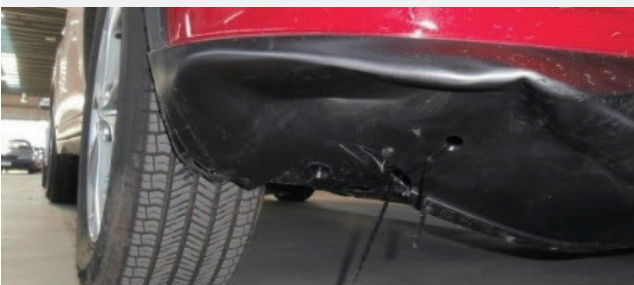
Deformation / major impact damage
