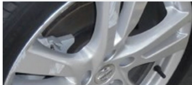
Major scuffing on wheel greater than 10% of surface area
