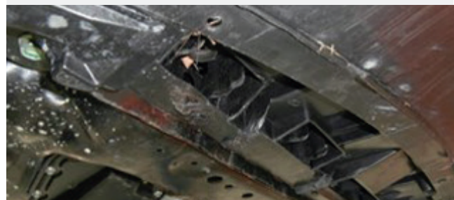
Deformation / major impact damage
