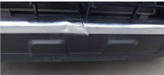
Cracked and dented bumper and grille
